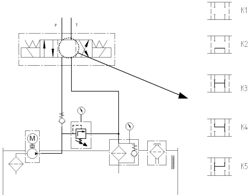
Suitable for single-acting cylinders to operate such as feedings, positional units, press rollers, presses, clamping units, etc. The effect of the type of middle position:
