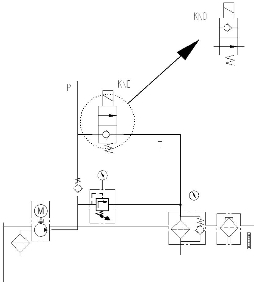
Suitable for single-acting cylinders to operate such lift tables, presses, etc. It has got excellent position holding parameters, because the seat valves has got minimal leakage. Normally closed (KNC – pressure on the P output) and normally open (KNO) type.
